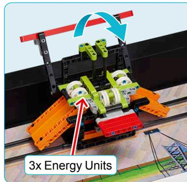
Load three energy units and lower the red bar as shown.
